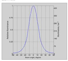
\* Illuminance is measured at a distance of 6.7m. For additional information refer to Lux diagram.
