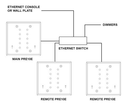
Data transport between each sACN capable device takes place using standard Ethernet hardware that supports multicast traffic. The above diagrams utilize a single Ethernet switch for simplicity. Any network hardware constituting a properly configured LAN may replace the Ethernet Switch blocks above.
